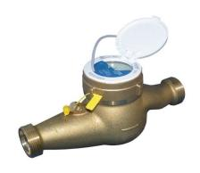
The Elster M190 is a multi-jet warm water meter with a dry register. It operates on the velocity principle in which water enters the measuring chamber through a number of ports and drives the inner rotor. This movement is transmitted by a magnetic coupling to the register which displays the total quantity passed.
