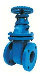
A cast iron, full bore gate valve with a bronze trim conforming to BS3464. The higher pressure and temperature ratings gives this valve more flexibility on applications that it can be used on. It's particularly suitable for water and oil.
