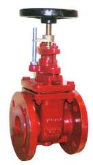
Good quality inside screw, non rising stem, non rising handwheel. Suitable for cold and hot water, seawater, saturated steam, oil and other neutral non aggressive liquids.
