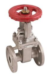
The JV060039 is a stainless steel, full bore, non-rising stem gate valve with a stainless seat, wedge and stem ideally suited for water distribution, gas oil, steam petrochemical, petroleum industry and various other duties.
