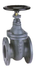
A economic PN10 rated cast iron, full bore gate valve with a brass seat and stem with PN6 drilled flanges ideally suited for water applications.
