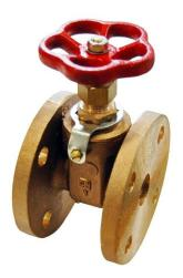
A marine gate valve with secured screwed bonnet, a non rising stem and a metal seat suitable for cold and hot water, seawater, oil and other neutral non aggressive liquids.
