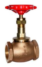
This robustly manufactured screwed bonnet globe valve with a metal valve disc is ideally suited for isolation duty, providing a leak-tight shut off with the capability of being used partially open to regulate flow.
