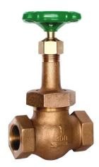
This robustly manufactured union bonnet globe valve with a stainless steel seat and disc configuration is designed for higher pressure and temperature isolation duty, providing a leak-tight shut off with the capability of being used partially open to regulate flow.
