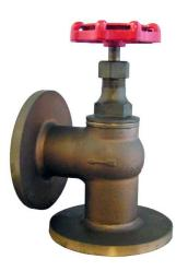
An economical angled pattern globe valve with a PTFE seat which is ideally suited for isolation duty, providing a leak-tight shut off with the capability of being used partially open to regulate flow.
