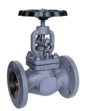
This bolted bonnet globe valve with a stainless steel valve disc has a non-return design, preventing reverse flow when in the open position. Also suitable for isolation duty, providing a leak tight shut off.
