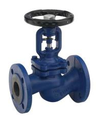
This bolted bonnet bellow sealed globe valve with a stainless steel valve disc is ideally suited for isolation duty, providing a leak tight shut off with the capability of being used partially open to regulate flow.
