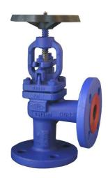
The 35.007 angled pattern bolted bonnet cast steel globe valve with a stainless steel valve disc has been pressure tested and witnessed by Lloyds Register of Shipping (LRS) and therefore ideally suited for shipside and marine boiler duty. Also suitable for many other applications where isolation of steam, gases and liquids is required.
