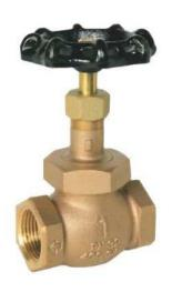
An economic union bonnet globe valve with a PTFE valve disc, ideally suited for isolation duties of sea water, steam and many other applications, providing a leak-tight shut off with the capability of being used partially open to regulate flow.
