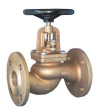
Bronze bolted cover, rising stem, metal seated gland packed globe valve. Suitable for cold and hot water, seawater, saturated steam, oil and other neutral non aggressive liquids.
