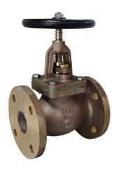
Bronze bolted cover, rising stem, metal seated gland packed globe valve. Suitable for cold and hot water, seawater, saturated steam, oil and other neutral non aggressive liquids.
