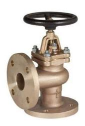
Bronze bolted cover, rising stem, metal seated gland packed globe valve. Suitable for cold and hot water, seawater, saturated steam, oil and other neutral non aggressive liquids.
