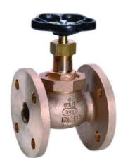
Bronze secured union bonnet, rising stem, metal seated gland packed globe valve. Suitable for cold and hot water, seawater, saturated steam, oil and other neutral non aggressive liquids.
