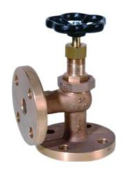
Bronze secured union bonnet, rising stem, metal seated gland packed globe valve. Suitable for cold and hot water, seawater, saturated steam, oil and other neutral non aggressive liquids.
