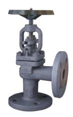
This bolted bonnet globe valve with a stainless steel valve disc has a non-return design, preventing reverse flow when in the open position. Also suitable for isolation duty, providing a leak tight shut off.
