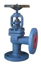
This bolted bonnet globe valve with a stainless steel valve disc is ideally suited for isolation duty, providing a leak tight shut off with the capability of being used partially open to regulate flow.
