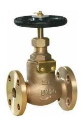
Bronze metal seated gland packed globe valve to JIS Japanese specifications. Suitable for cold and hot water, seawater, saturated steam, oil and other neutral non aggressive liquids.
