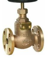
Bronze metal seated gland packed globe valve to JIS Japanese specifications. Suitable for cold and hot water, seawater, saturated steam, oil and other neutral non aggressive liquids.
