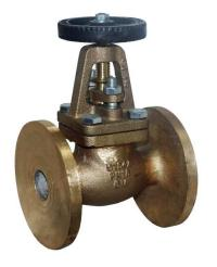
Bronze bolted cover, rising stem, metal seated gland packed globe valve. Suitable for cold and hot water, seawater, saturated steam, oil and other neutral non aggressive liquids.
