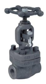
This JV060082 carbon steel class 800 globe valve is designed to API 602 and tested to API 598, it is suitable for high pressure and temperature duties
