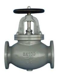
Cast steel metal seated gland packed globe valve to JIS Japanese specifications. Suitable for cold and hot water, seawater, saturated steam, oil and other neutral non aggressive liquids.
