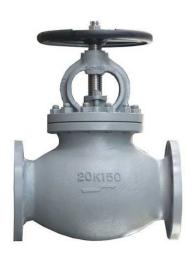
Cast steel metal seated gland packed globe valve to JIS Japanese specifications. Suitable for cold and hot water, seawater, saturated steam, oil and other neutral non aggressive liquids.
