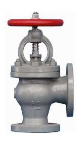
Cast steel metal seated gland packed globe valve to JIS Japanese specifications. Suitable for cold and hot water, seawater, saturated steam, oil and other neutral non aggressive liquids.
