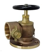
This angled pattern fire hydrant valve with screwed bonnet is suitable for both offshore and onshore applications. Constructed with a dual seat design, the primary valve seat is hard rubber with an additional secondary metal to metal seat.
