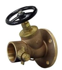
This straight pattern fire hydrant valve with screwed bonnet is suitable for both offshore and onshore applications. Constructed with a dual seat design, the primary valve seat is hard rubber with an additional secondary metal to metal seat.
