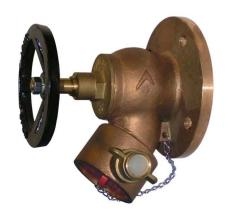
This oblique pattern fire hydrant valve with screwed bonnet is suitable for both offshore and onshore applications. Constructed with a dual seat design, the primary valve seat is hard rubber with an additional secondary metal to metal seat.
