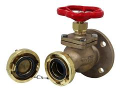
Marine grade bolted bonnet fire hydrant valve suitable for both offshore and onshore applications. Constructed with a dual seat design, the primary valve seat is NBR with an additional secondary metal to metal seat.
