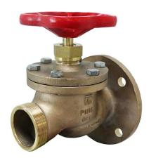
Marine grade bolted bonnet fire hydrant valve Approvals, Features & Benefits suitable for both offshore and onshore applications. Constructed with a dual seat design, the primary valve seat is NBR with an additional secondary metal
