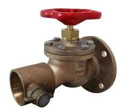
Marine grade bolted bonnet fire hydrant valve suitable for both offshore and onshore applications. Constructed with a dual seat design, the primary valve seat is NBR with an additional secondary metal to metal seat.
