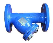
The JV150022 is an economical WRAS approved cast iron Y type strainer with a stainless steel screen, ideally suited for potable water applications to protect meters, pumps, valves and other pipeline equipment.
