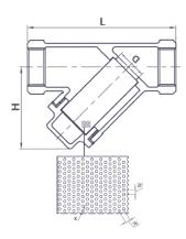
The JV150023 is a WRAS approved Y-type strainer with a stainless steel screen ideally suited for water applications to protect meters, pumps, valves and other pipeline equipment.
