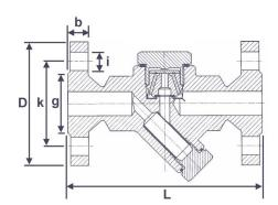
The JV160002 thermodynamic steam trap is manufactured and tested in accordance with the DIN standards and the relevant German regulations for steam boilers (TRD) and pressure vessels (AD).
