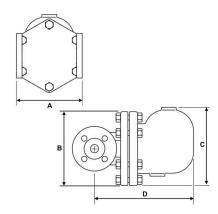
The JV160006 is a float type steam trap for draining condensate in steam lines. This steam trap is capable of draining large capacities of condensate and is well adapted to the changes of flowrates.
