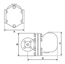
The JV160008 is a float type steam trap for draining condensate in steam lines. This steam trap is capable of draining large capacities of condensate and is well adapted to the changes of flowrates.
