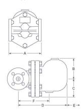
Manufactured by Spirax Sarco, the FT43 is a maintainable ball float steam trap with integral automatic air venting facility.
