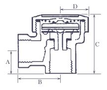
Manufactured by Spirax Sarco, the AV13 is a maintainable balanced pressure thermostatic air vent with angled connections.
