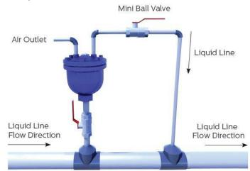
As the air is discharged from the system into the atmosphere, the liquid is reintroduced into the system by the JV170004
