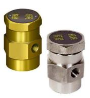
The JV170006 vacuum breaker is used on steam Approvals, Features & Benefits systems and heat exchangers. When these are turned off they still contain a certain amount of steam. The steam condenses as the vessel cools down and since condensate occupies a much smaller volume than steam, vacuum conditions are generated.
