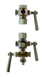
The JV190004 set of gauge cocks are fitted with sleeves which can be adjusted by means of packing nuts as wear necessitates, providing easy and efficient maintenance.
