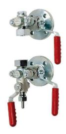
The JV190006 set of gauge cocks are fitted with sleeves which can be adjusted by means of packing nuts as wear necessitates, providing easy and efficent maintenance.
