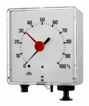
The **JV190019P** is for use with tanks which have a height or vertical diameter of up to 3 meters and containing most liquids with a viscosity of up to 200 secs. Redwood No.1 i.e. light heating oils, water, etc. These gauges are always works preset and calibrated to your requirements.
