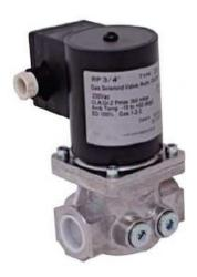
The JV230001 is a Class "A" gas solenoid valve suitable for gas in gas power burners, atmospheric gas boilers, industrial ovens and other gas consuming appliances.
