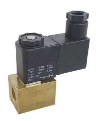
The JV230010 is a small bore direct acting general purpose solenoid valve suitable for air, water and light oils up to 40 centistokes.
