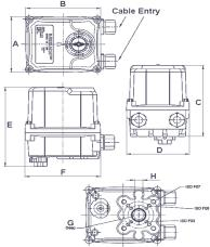
HQ-L Electric 1/4 Turn Low Torque Actuator 40Nm - 60Nm
