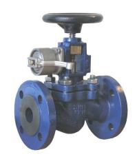
In the event of emergency or dangerous situations, quick closing valves quickly shut-off of pipe line systems carrying combustible liquids. They operate by means of remote control from outside the danger area. Under normal circumstances they are in an open position.
