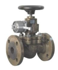
In the event of emergency or dangerous situations, quick closing valves quickly shut-off of pipe line systems carrying combustible liquids. They operate by means of remote control from outside the danger area. Under normal circumstances they are in an open position.
